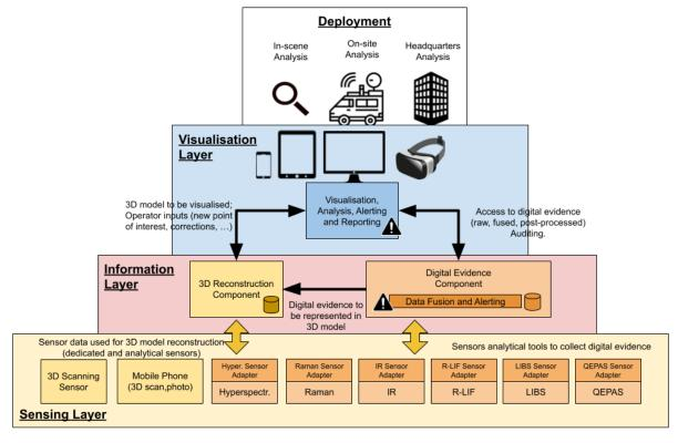
Figure 1 - RISEN system layers
