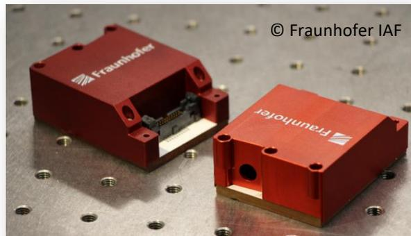
**Figure 2.** Miniaturized, broadband spectrally tunable MOEMS EC-QCLs with emission wavelengths in the mid-infrared range and high scanning frequency up to 1 kHz. Such tiny, palm-size devices are developed at the Fraunhofer Institute of Applied Solid State Physics (IAF) in collaboration with the Fraunhofer Institute for Photonic Microsystems (IPMS).
