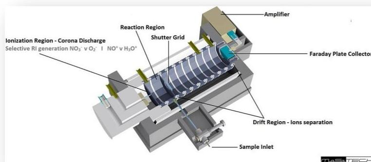
Figure 4. Schema of IMS.
