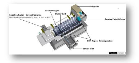
Figure 4. Schema of IMS.
